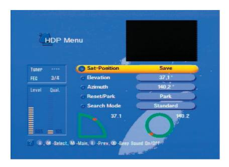
Use the keys to go to the "Reset/Park" option, and change the selection to "Reset" using the keys. Now press The following screen appears:
